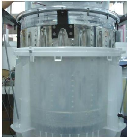
Figure 12. Washing unit for fluid flow visualization and PIV experiments.
