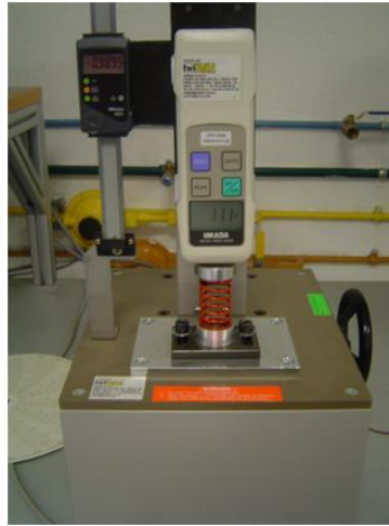
Figure 16. Suspension coil spring stiffness measurement.
